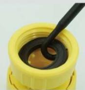
\*Removing / manipulating O-rings, small seals / gaskets, clips. Cleaning air vent assemblies.
