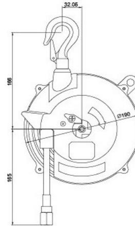
Hose Balancer (Air tool balancers) are Designed for Small Pneumatic Tools.
