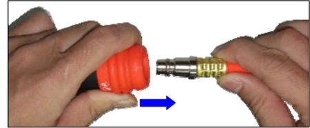
2st Step : Push Forward - Disconnect the air nipple
