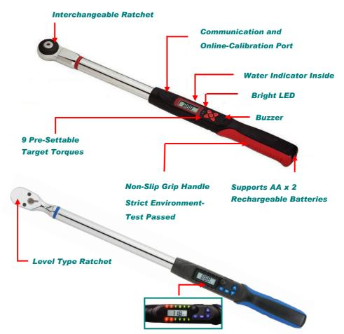
When approaching the target torque, the green lights will illuminate (a warning signal). When the target torque has been reached, the red lights will illuminate (a stop signal).
