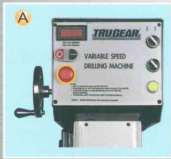
■ 24V Control Panel, LED readout
